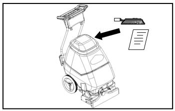
STEP 1 Remove electrical cord and literature from recovery tank. Fill solution tank (see filling instructions page 6).
